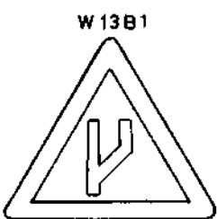
W 13B1 BEGINNING OF DUAL ROADWAYS
